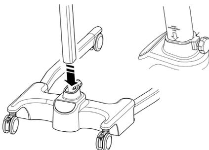
3. Tighten the mast assembly with the mast-locking device, which is located at the front of the chassis.
