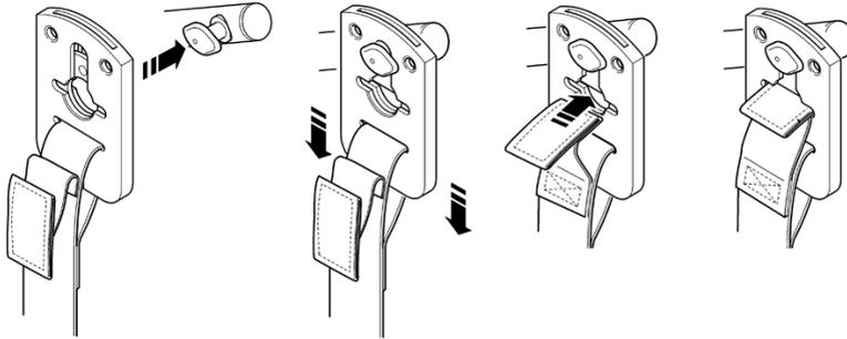
Securi3 sling attachment system. Example of installation.
