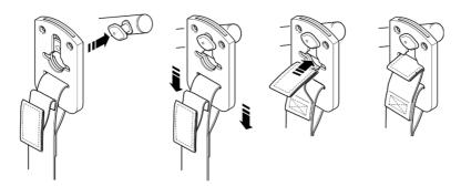
Securi3 sling attachment system. Example of installation.
