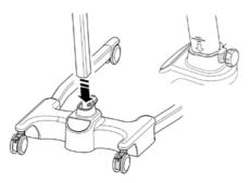
**3.** Tighten the mast assembly with the mast-locking device, which is located at the front of the chassis.
