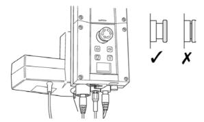
• Push the up and down buttons on the hand control to confirm that the boom rises and lowers satisfactorily.
