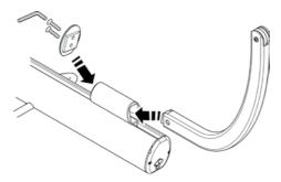
Attach four point positioning cradle to the lift boom by inserting the split pin. Ensure pin is secure.
