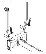
3. Using Allen Key provided, tighten the 6mm screws located on each side of the chassis.
