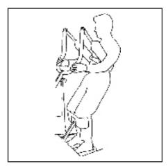
Position Standaid so that the client's feet fit in the foot trays and knees rest against the knee pad. Initially attach the longer loops of the sling to the white hooks at the end of the hand grips. The client's hands should be placed on the black hand grips or support handles. (Once the client is used to the lift, the shorter loops may be used to achieve a more upright position). Then push the up button on hand control to raise the client to the standing position.
