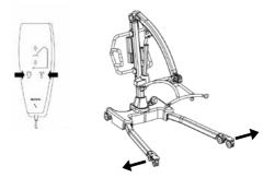
• Push the up and down buttons on the hand control and confirm the boom rises and lowers.
