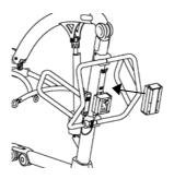
**9.** Plug the handset and actuator cables into the bottom of the controller. Refer to the figures on page 12 or 13 for correct positions.
