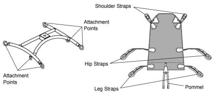
6-point cradle. Example of the 6-point cradle sling with loop attachments.
