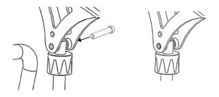
7. Insert the quick-release pin through the quick-release pin sleeve until it is fully located.
